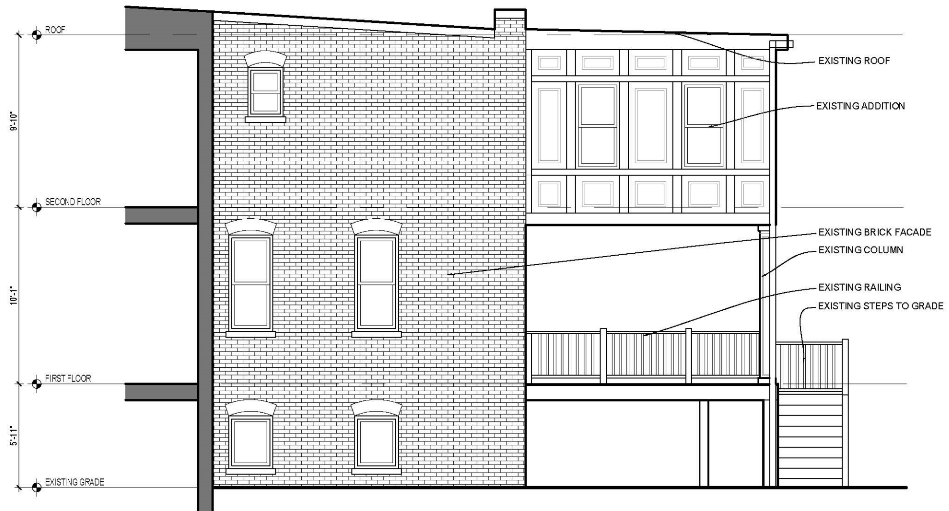
1 EXISTING NORTH ELEVATION D-4 SCALE: 3/16"=1'-0"
